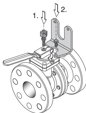
3. Attach the upper part of the mounting bracket with the sensor plate to the previously assembled base. The bore holes allow a rough height adjustment.
